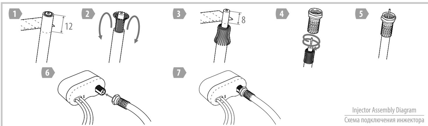
Injector Assembly Diagram
