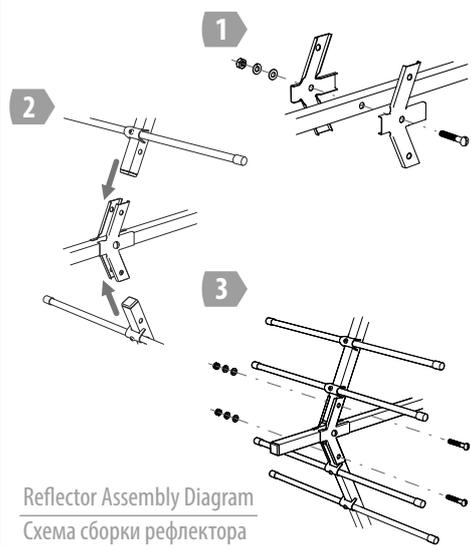
Reflector Assembly Diagram
