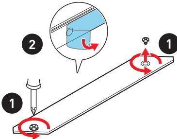
3. Move and fasten the M.2 standoff to the appropriate position for your M.2 SSD, or remove the M.2 standoff if your M.2 SSD length is same as the length of M.2 heatsink to avoid damage to the M.2 SSD.
