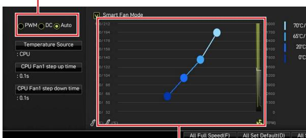
There are gradient points of the fan speed that allow you to adjust fan speed in relation to CPU temperature.
