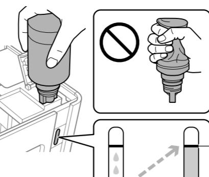
Ink flow stops automatically when the ink level reaches the upper line.
