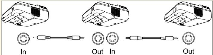
The diagram shows a sequence of three projectors connected in a chain. The first projector's SYNC OUT port is connected to the second projector's SYNC IN port. The second projector's SYNC OUT port is connected to the third projector's SYNC IN port. Labels 'In' and 'Out' are placed under the respective ports.
