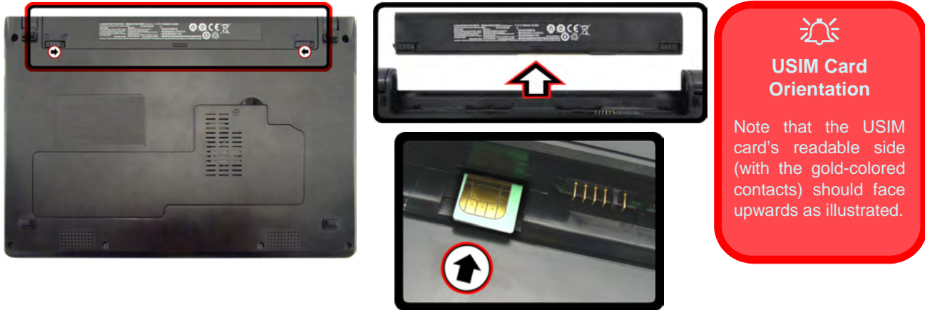
Figure 1 - 9 - Battery Removal & USIM Card Insertion
