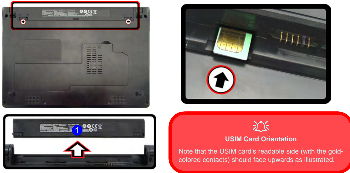
Figure 6 - Battery Removal & USIM Card Insertion
