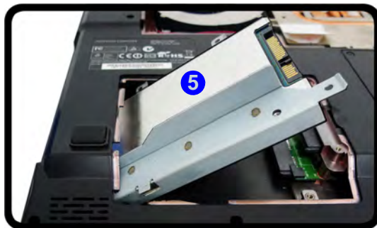
Figure 6 - 9 Secondary HDD Assembly Removal (Model C)
