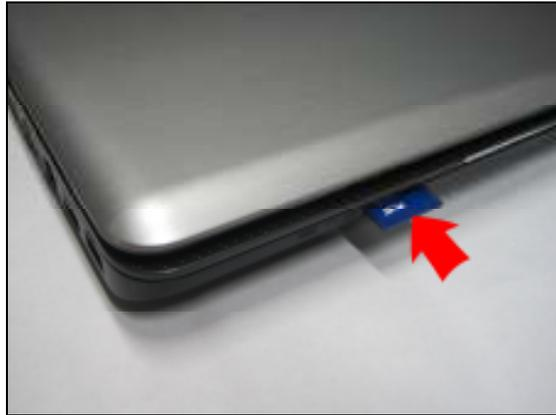
Hold the SD/MMC/MS card with its orientation symbol pointing into the slot and the topside of the card facing up.
