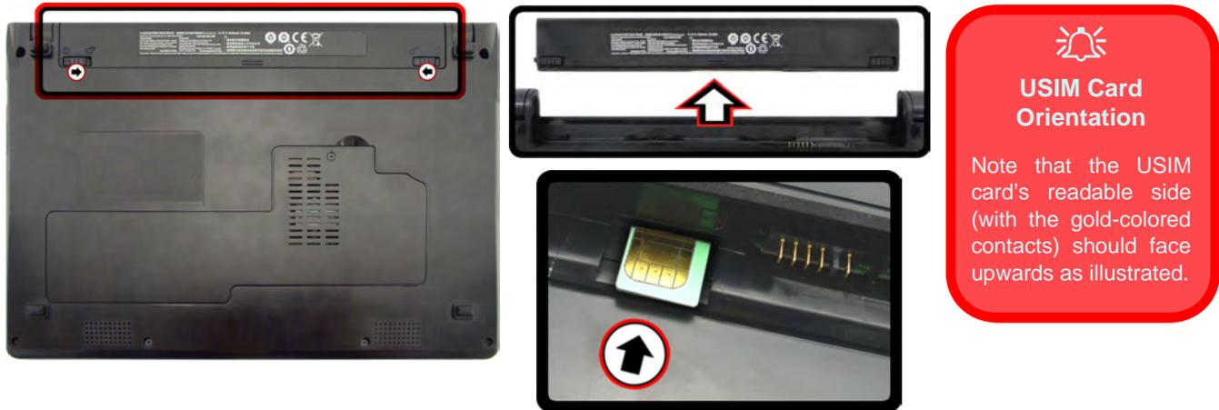
Figure 1 - 9 - Battery Removal & USIM Card Insertion
