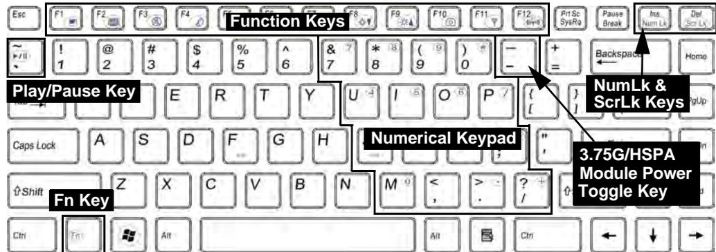
Figure 1 - 8 - Keyboard - Model A Design III
