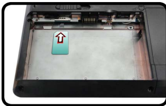
Figure 19 - Remove the battery and Insert the USIM Card
