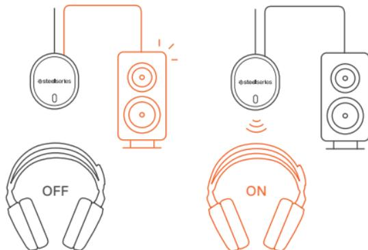
When headset is off, audio can be sent to speakers via Line Out. When headset is powered on Line Out is automatically muted.
