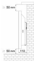
Figure 9. Dimensions of the convector after assembly
