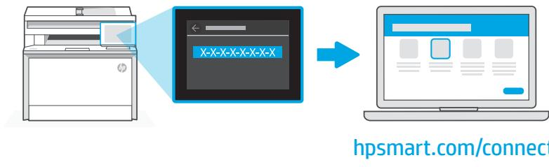
**EN** 1. Record the pairing code that displays on the control panel. The pairing code will expire after a limited time. If code expires, generate a new code in HP Easy Start.
