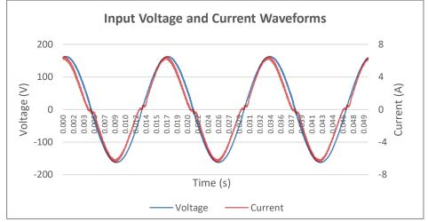
Input AC Current Waveform (ITHD = 12.46%, 50% Load)
