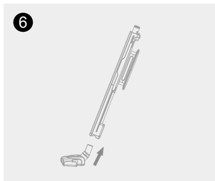
6. Keep the brush aligning the interface of the connecting tube, insert it slowly.
