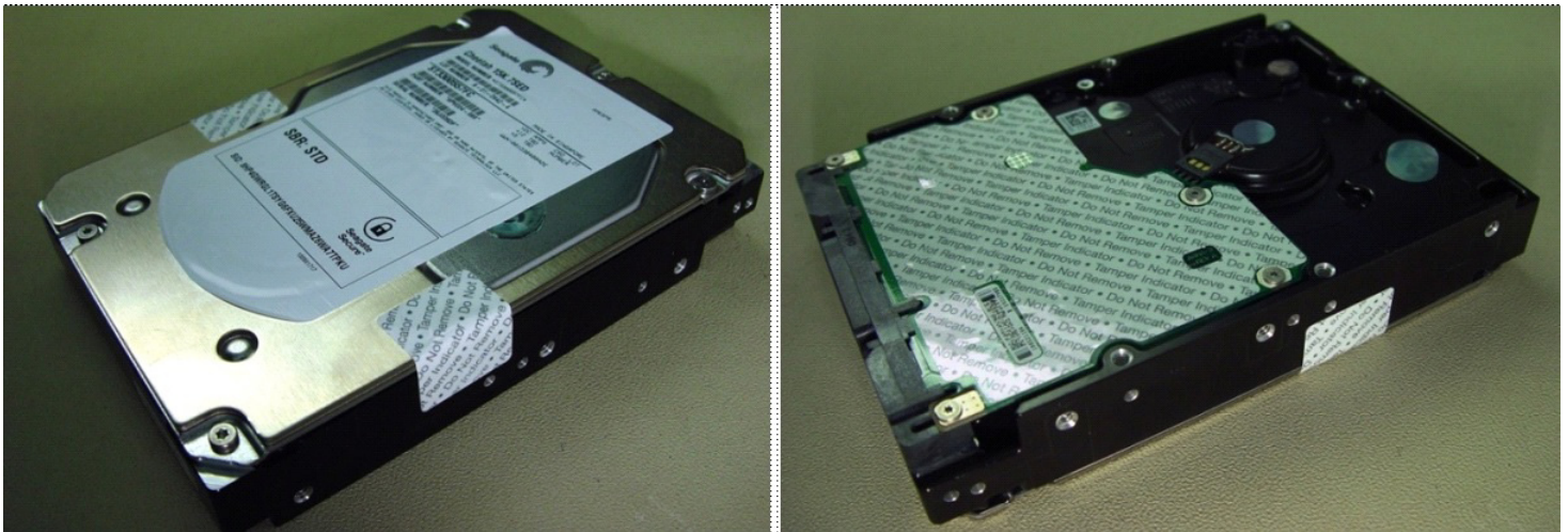
Figure 6. Example of FIPS tamper evidence labels.
