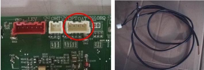
**Solution:** Check the connector of sensor and slot, if loose or not plugged in, please connect again.
