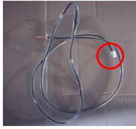
**Solution:** Check the connector of sensor and slot, if loose or not plugged in, please connect again.
