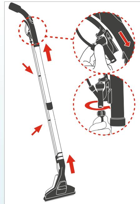
**If using the upholstery spray nozzle, connect this directly to the handle of the suction hose.**
