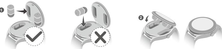
1 Attach the earbuds directly to the inside of the watch cover, with the ear tips facing downwards.
