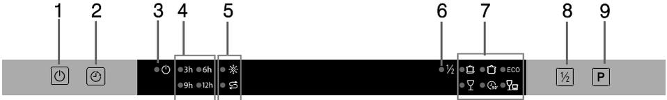
1. On/Off Button: To turn on/off the power supply.
